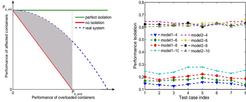
**Fig. 1.** Isolation curve including perfect isolation, no isolation and real system isolation. **Fig. 2.** Performance isolation with different workload of well-behaving containers.
