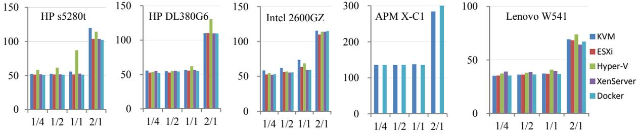
**Fig.2** Completion time of varying computing workloads (x axis: workload level, y axis: completion time ( $10^3$  seconds))
