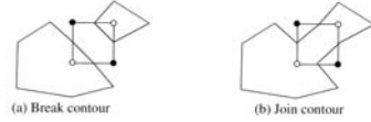
Figure 6-8 Choosing a particular contour case will break (a) or join (b) the current contour. Case shown is marching squares case 10.
