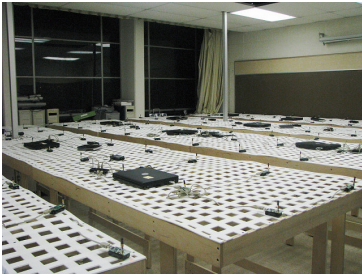
Fig. 4. NetEye wireless sensor network testbed.
