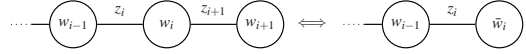
Figure 3. The reduction of processors P_i and P_{i+1} to a single equivalent processor.
